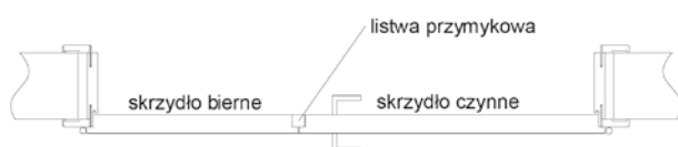
DOUBLE DOOR SYSTEM. PASSIVE LEFT, ACTIVE RIGHT
